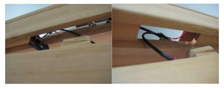
Note: Position the cam locks on the top of the Left & Right Wall panels as shown above.
