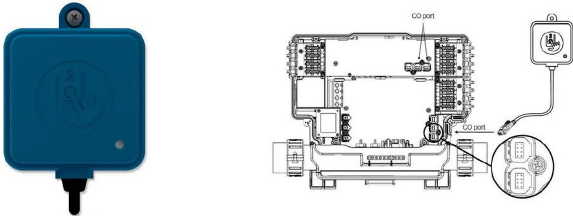
The in. touch 2 spa transmitter must be installed under the spa skirt, at least 12" (30 cm) away from any metal component or structure, as close as possible to the house to optimize the signal strength.
